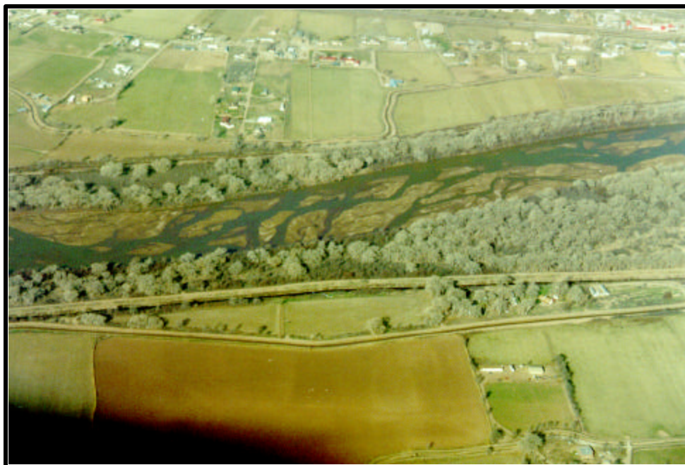
Plate A.16. View of Rio Grande between Isleta and Belen at about RM 164. Note the presence of bank-attached alternate bars and mid-channel braid bars.
