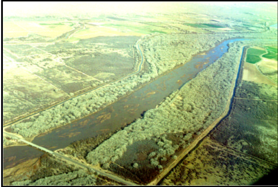
Plate A.19. View of Rio Grande at the US Highway 60 Bridge near Bernado (RM 130.6). The USGS gaging station is located at this bridge. Note the presence of numerous braid bars in the channel.
