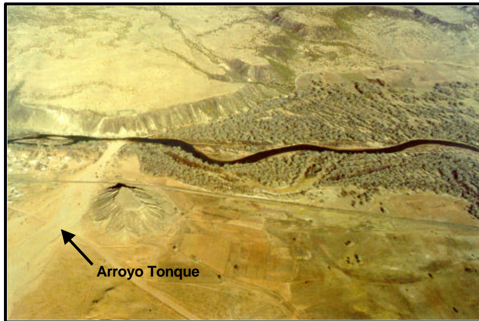
Plate A.6. View of Rio Grande at San Felipe Pueblo and Arroyo Tonque confluence at RM 216.2. The valley constriction formed by the bedrock outcrop and alluvial fan at San Felipe is the boundary between geomorphic Subreaches 1 and 2. Note the absence of unvegetated bars upstream of the confluence.
