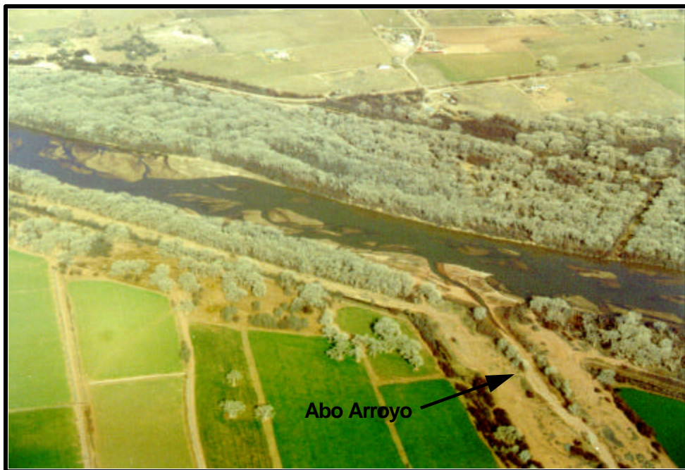
Plate A.18. View of Rio Grande at the confluence of Abo Arroyo at RM 139.2. Note the tributary mouth bar that has built out into the Rio Grande and the presence of numerous braid bars in the channel.
