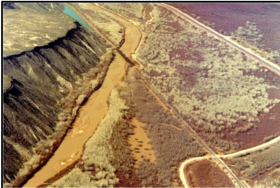
Plate A.34. View of the Rio Grande at the San Marcial Railroad Bridge and USGS gaging station at about RM 68.6. The reach is actively aggrading due to the backwater effects of Elephant Butte Reservoir. Note the extensive braid bars in the channel.
