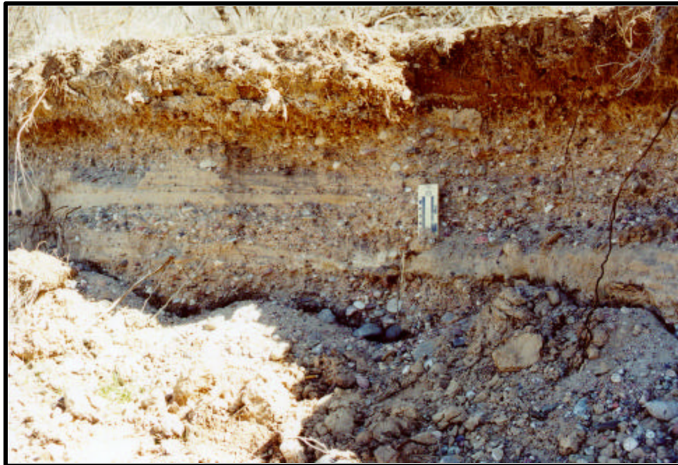
Plate A.4. View of bank stratigraphy at Pena Blanca (RM 227). Note the interbedded sands and gravels that reflect the caliber of the sediments that were being transported by the river when the floodplain was formed.
