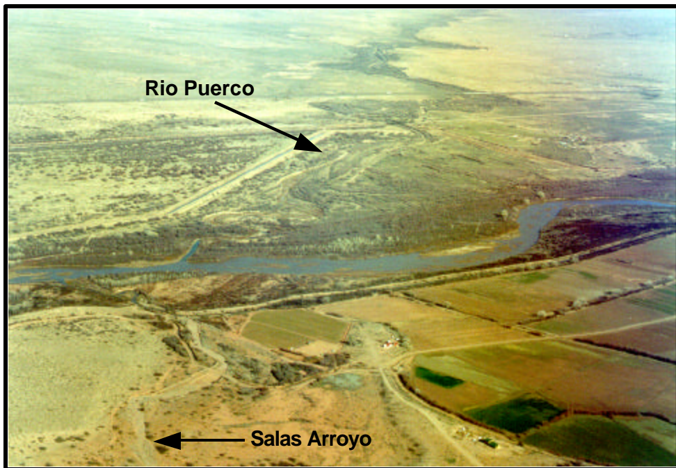
Plate A.20. View of Rio Grande at the confluences of the Rio Puerco and Salas Arroyo at about RM 126.8. Numerous braid bars are present in the channel upstream of the confluences.
