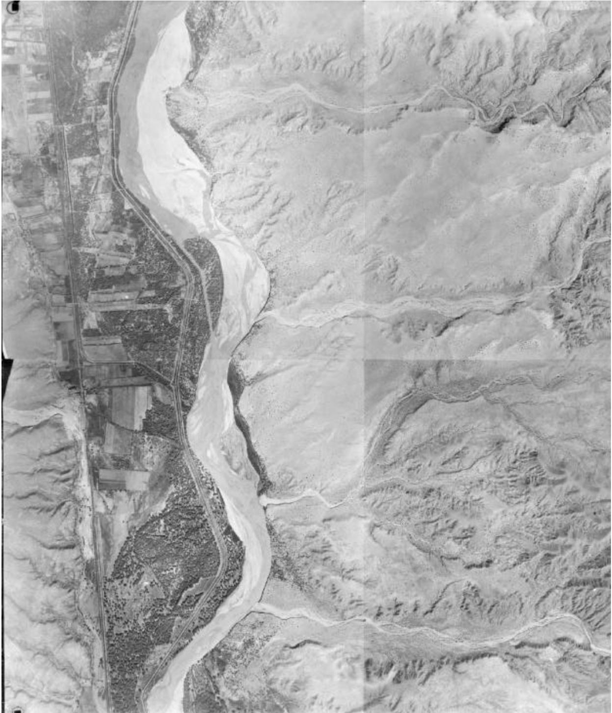
Figure 3.4. 1935 aerial photograph (#5925A) showing the high frequency of east-side tributary arroyos draining the Joyita Uplift in Reach 6, and delivering sediment to the Rio Grande. The reach of the river is located near Socorro, between RM 96 and RM 102.
