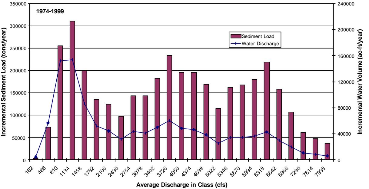
Figure 3.71. Histograms of incremental bed-material load by discharge class for the pre- and post-Cochiti Dam periods at the San Felipe gage. Also shown is the incremental water volume within each discharge class.
