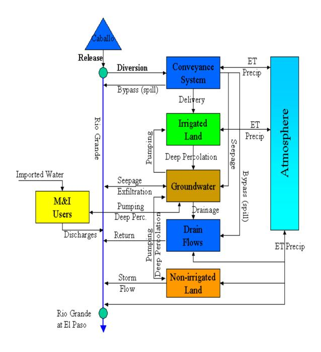
Figure 8.1: Hydrologic Schematic of the Rio Grande Between Caballo Dam and Courchesne Bridge (Rio Grande At El Paso Gauging Station).
