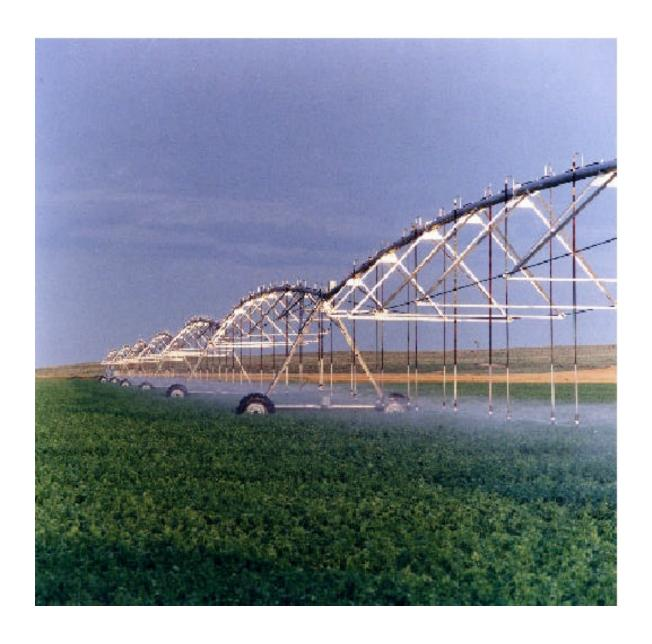
Figure 8.2: Center Pivot Irrigation System (from Zimmatic, Inc.).
