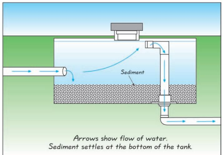
Figure 8-10: Example of a sediment trap. The top photo shows the installation of two traps; the illustration depicts how water flows through a trap.
