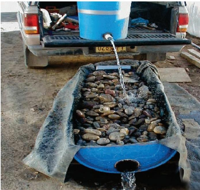
Figure 8-4. An above ground demonstration of how a funnel drain works. Materials, shapes and proportions of funnel drains can vary.
