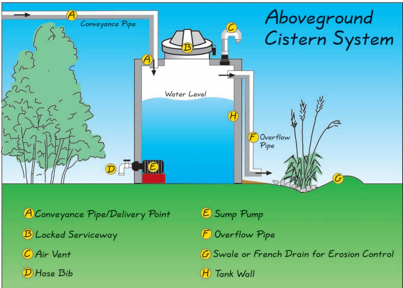
Figure 9-4: A “cutaway” drawing of an aboveground cistern system
