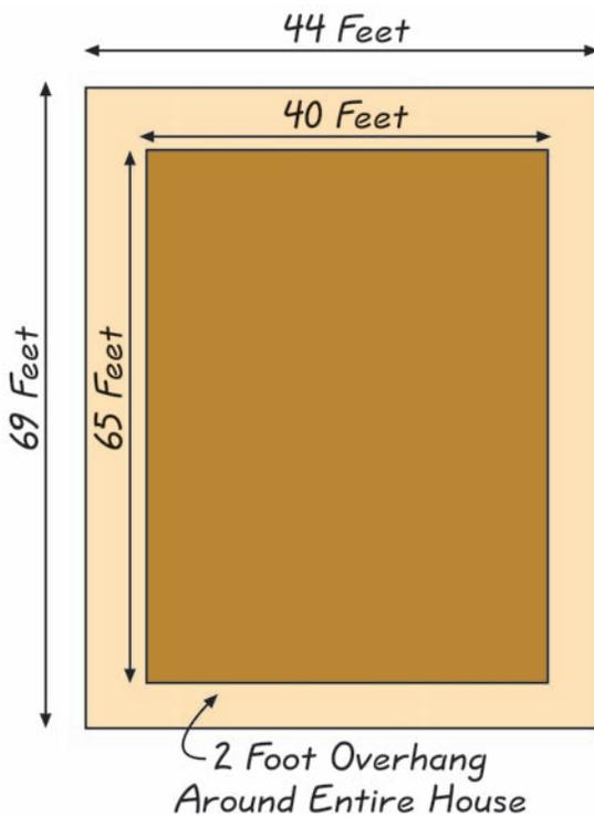
Figure 3-3: Calculating the catchment area including roof overhang
