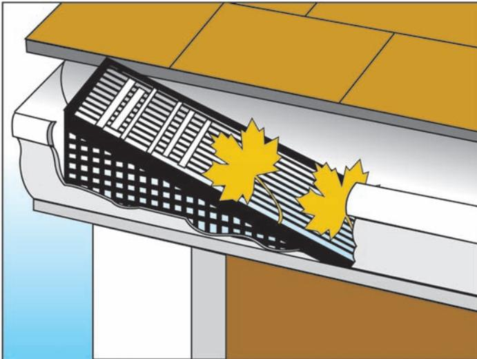
Figure 8-9: A leaf screen used as a method of filtration
